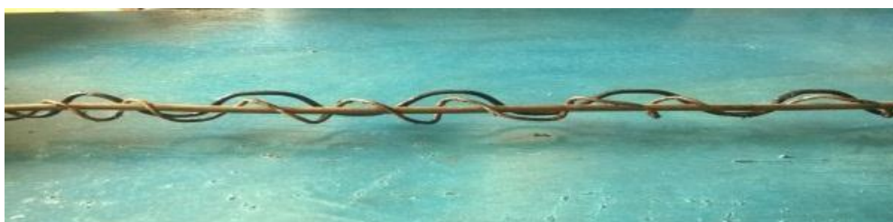
Fig. 5 Combination of screw and wire Insert
